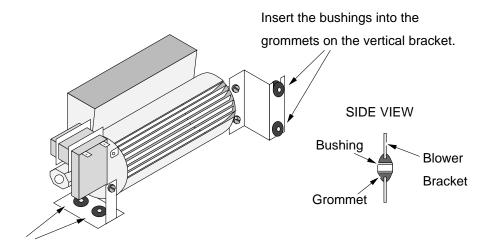
Make sure these two grommets are in place (they insulate the fireplace from blower vibration).
